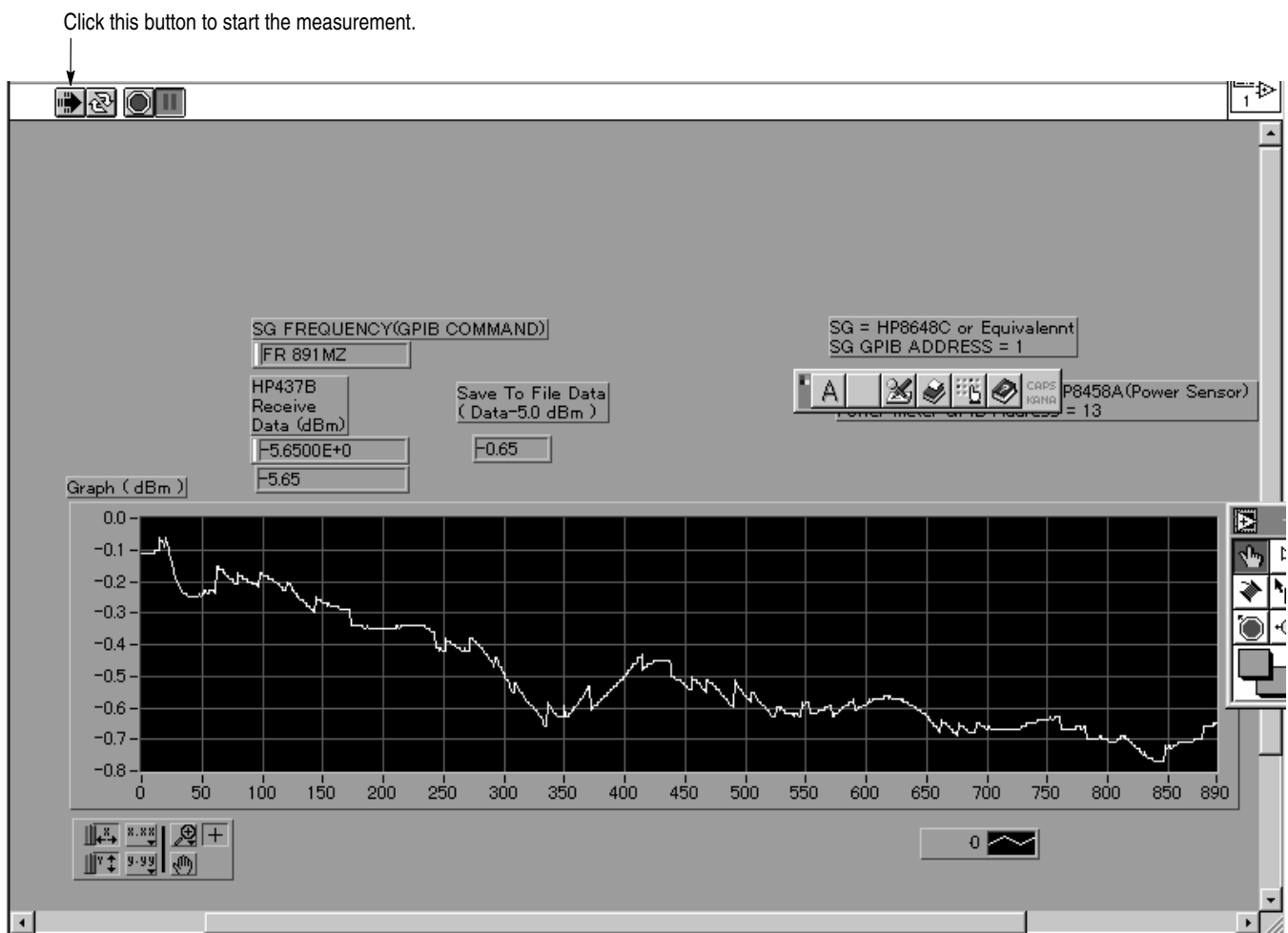
Figure 5–13: Running the SG flatness measurement program on PC
